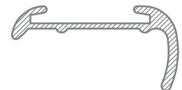
UA10622 31.75mm x 16.25mm Caravan J Mould 0.218 kg/m
