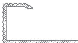
UA4414 13mm Serrated Capping 0.224 kg/m
