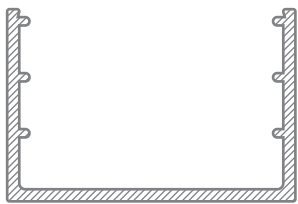
UA2096 38.10mm x 25.40mm Handrail Channel 0.394 kg/m
