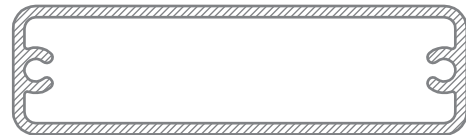
UA7613 60mm x 17mm Fence Panel 0.647 kg/m
