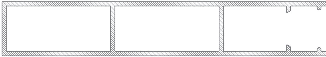
UBO25150 25mm x 150mm Batten Outer 2.009 kg/m
