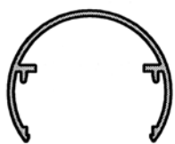
60mm \phi HANDRAIL UB006
