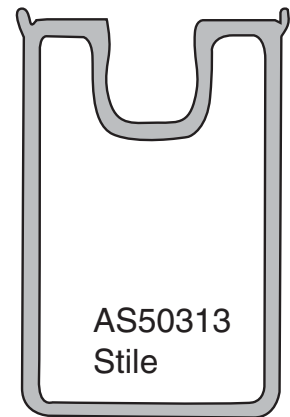
AS50313 Stile WT = 1.151kg/m AP = 228mm PP = 183mm
