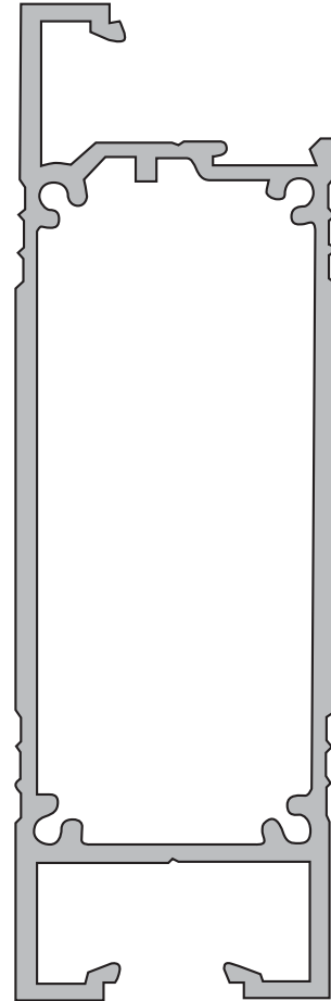
AS806 MID RAIL 136mm WT = 2.122Kg/m AP = 490mm PP = 300mm
