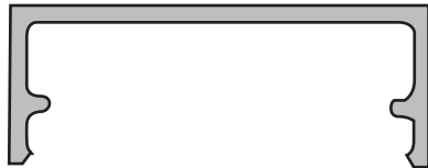
AS 7770 Snap Adaptor WT = 0.366 kg/m AP = 188mm PP = 100mm
